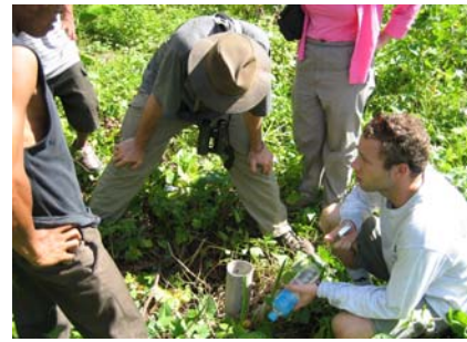
Figure 3: Performing a "perk" test
